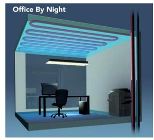
During the night the concrete core of the ceiling slab is cooled by the free cooling source or the chiller.
