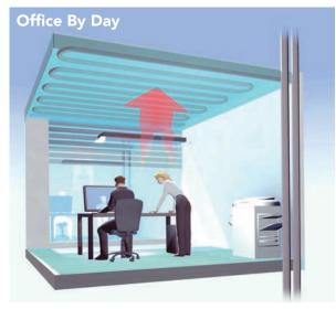
During the day the cooled ceiling slab accumulates the thermal loads from the room or direct sunshine.
