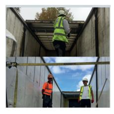
The lorry driver will open the rear doors and roof of the trailer. A ratchet strap will be placed across the opening to provide protection from falling.
